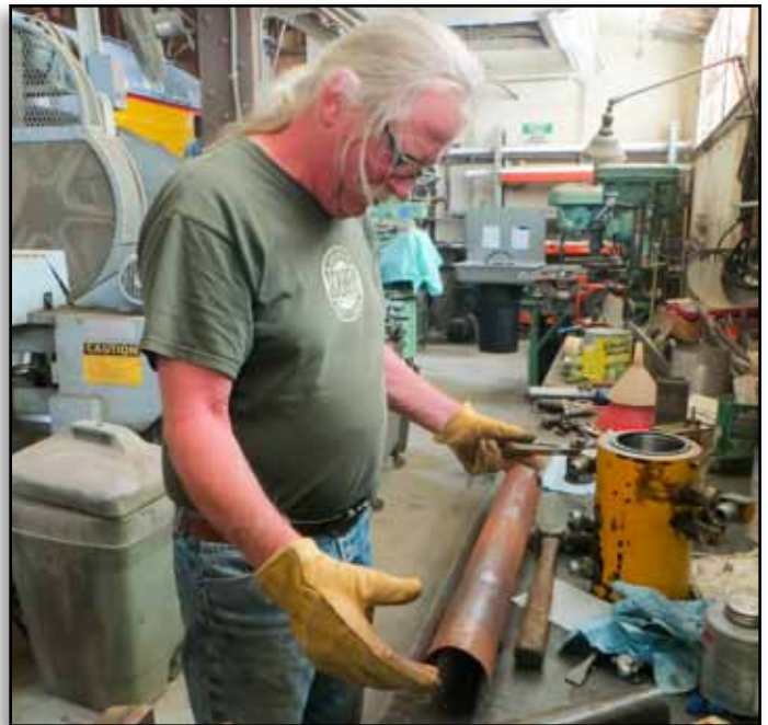
Earl Soladay fabricating an exhaust shroud for one of the gang cars. Ron Hyatt
